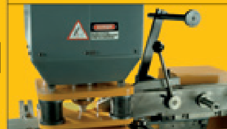
Optional 'drive-in' minimum deform stripper and bolster assemblies.
